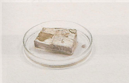
Figure 1.2 A freshly cut piece of sodium with a shiny surface. A few minutes later the surface has corroded.
