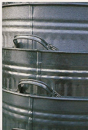
Figure 2.2 The dustbins and the cars are both protected from corrosion by zinc coating
